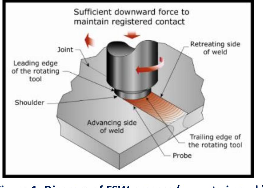
Figure 1. Diagram of FSW process (www.twi.co.uk)
